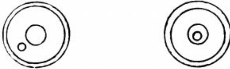
A right angle prism, or mirror, is usually mounted over the circular bubble vial to allow the instrument person to observe the bubble from his normal operating position. The bubble need only be inside the circle etched in the center of the circular vial for the instrument to operate satisfactorily. Thus the instrument person does not have to go through the time consuming procedure of precisely leveling the telescope tube as required for the Wye and Dumpy Levels.
