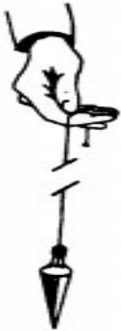
The importance of having both ends of the chain at the same elevation when measuring a horizontal distance cannot be over emphasized. One of the most common errors in chaining is failure to hold both ends of the chain at the same level.
