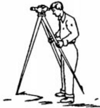
An accepted method of setting up the level is to place one tripod leg on the ground while holding the other two as shown in the above photo, and by using a fashion as to make the tripod head nearly horizontal. The tripod legs should be pressed firmly into the ground for added stability, remembering that the more nearly leveled the tripod head is kept the less the leveling screws on the instrument will have to be turned
